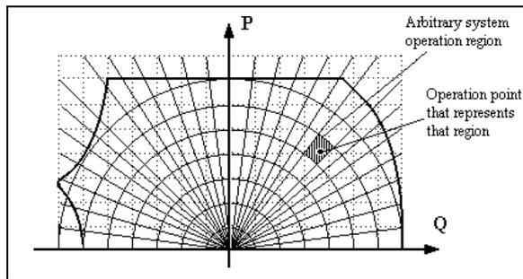
Fig.1 - Regions in the  $P \times Q$  plane used to design the GSPSS
