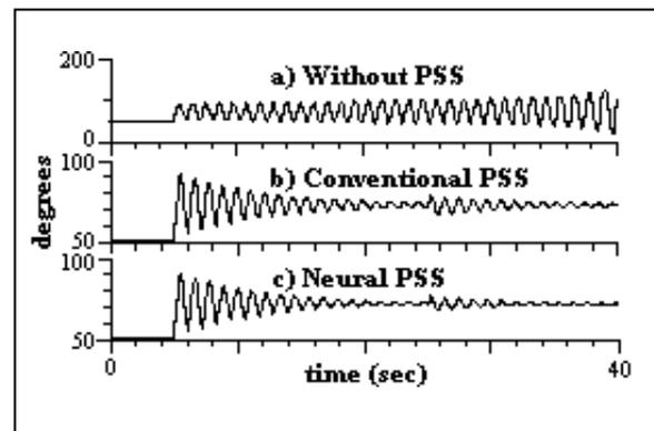
Fig.8 - Rotor angle (in degrees) for Case 1
