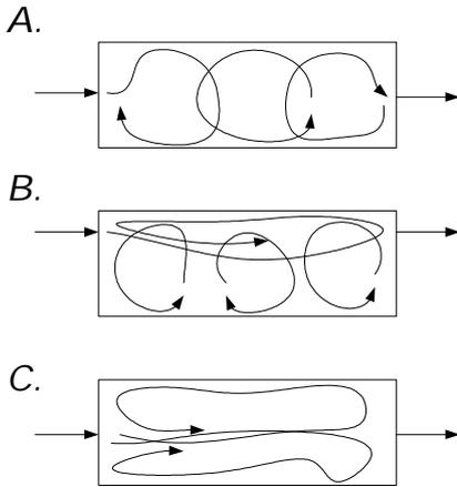
Figure 3: Typical side-viewed mixing patterns: A. catenary, B. mammillary and C. interconnected parallel.
