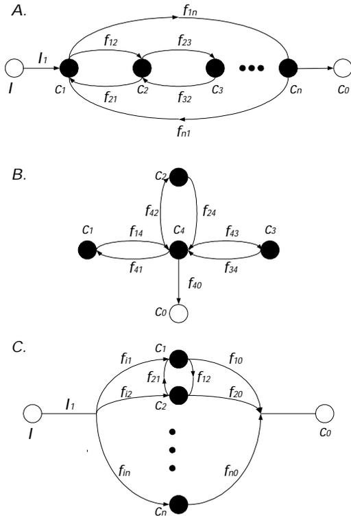
Figure 2: Elementary compartmental systems: A. circular/catenary, B. mammillary and C. interconnected parallel.
