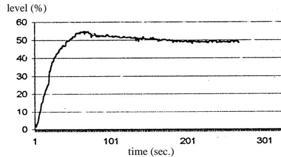
Fig. 6. Plant response using Ziegler-Nichols tuning procedure
