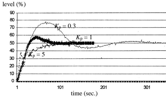
Fig. 4. Plant response to a step input of 50%
