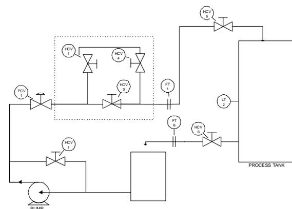
Fig 3. Process flow diagram of the mini-plant to be controlled
