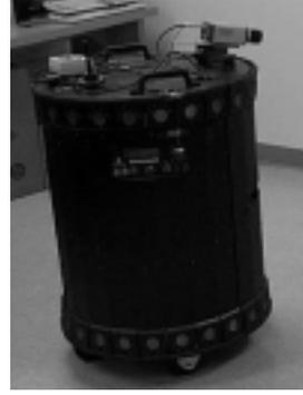
Fig. 1. The mobile robot with a laser range finder.
