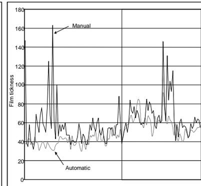
Fig. 10. Manual and automatic data superimposed. The data are shown in its index order of gathering.
