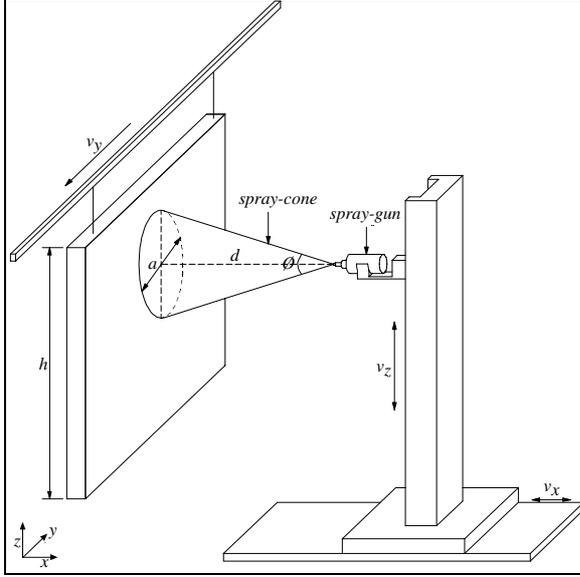
Fig. 3. Figure shows: a)-spray-painting task geometry assuming a plane surface; b)-spray-cone model as a simplified model of the powder spray cloud.
