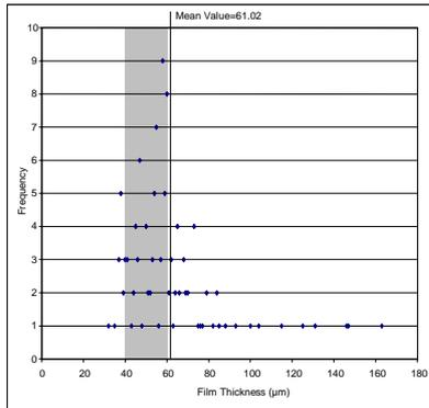
Fig. 8. Film thickness frequencies for manual painting.
