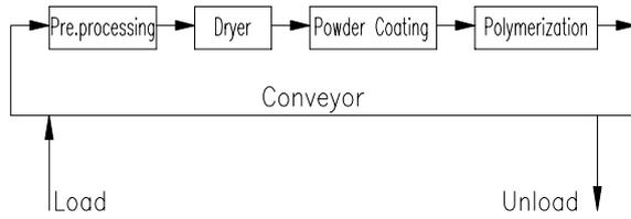
Fig. 1. Sequence of phases of a powder coating system.
