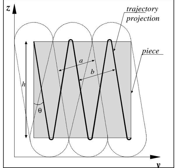
Fig. 4. Painting trajectory: the rectangle represents the workpiece surface and in the same figure is superimposed the spray-gun trajectory. In the figure is shown the particular situation in which the spray projection diameter is equal to the path width:  $a = b$ .
