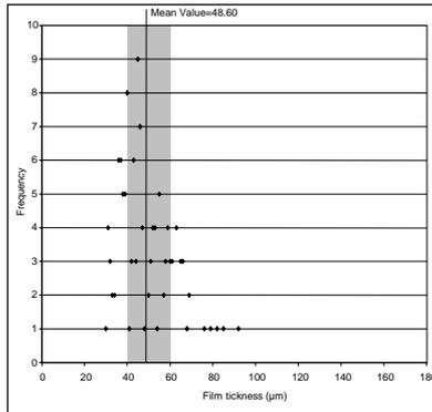
Fig. 9. Film thickness frequencies for automatic painting.
