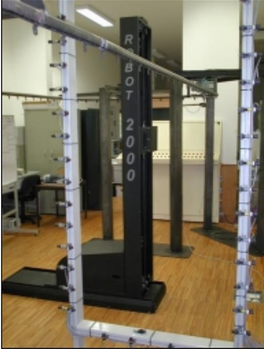
Fig.2. An EP-Robot prototype in a laboratory environment with an aerial conveyor to completely simulate the motions involved in the spray-painting.
