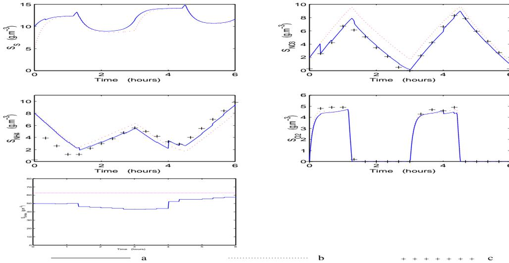
Fig. 2. Experiment 2. State estimation with EKF: estimates, **a**; nonlinear model, **b**; measurements, **c**.
