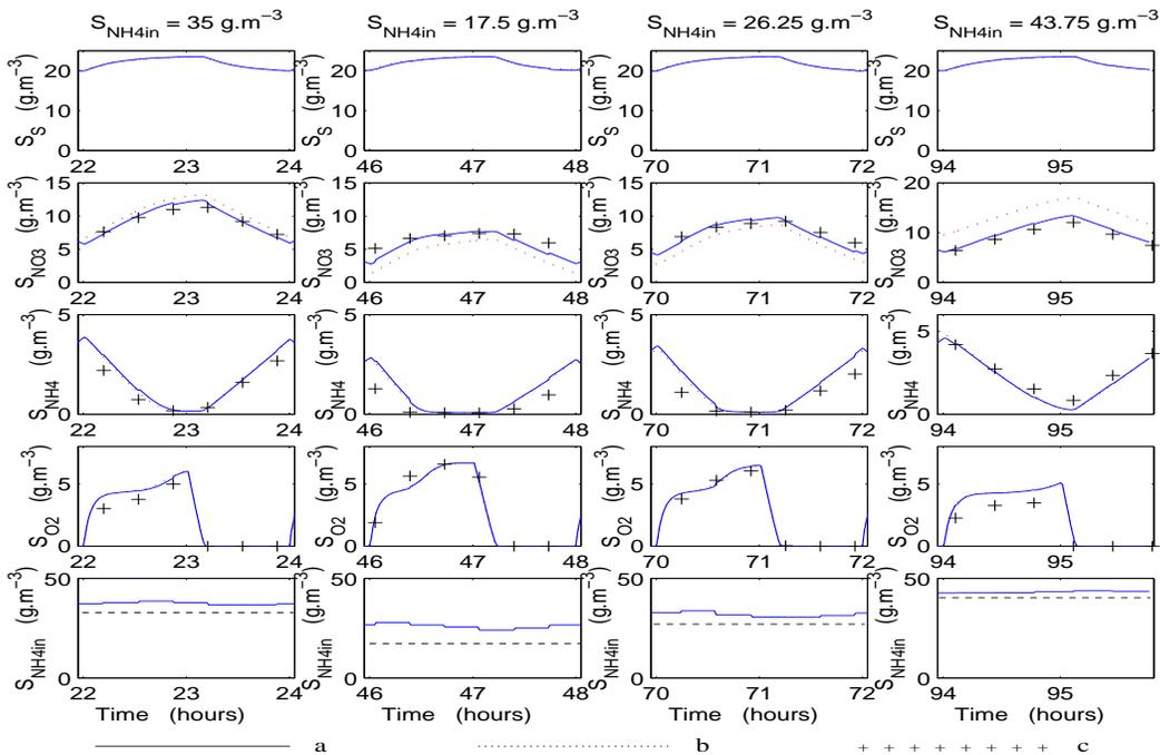
Fig. 3. GPSX data. State estimation with EKF: estimates, **a**; nonlinear model, **b**; measurements, **c**.
