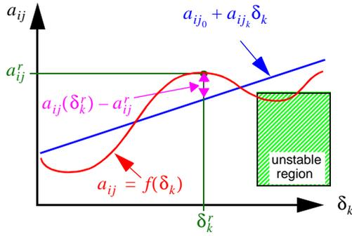
Fig. 2 Dependence of a matrix element on a parameter
