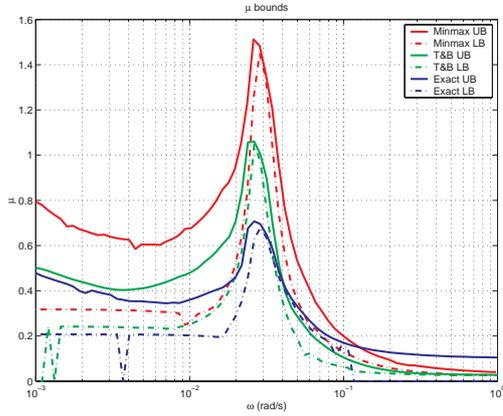
Fig. 3  $\mu$  bounds for the civil transport aircraft
