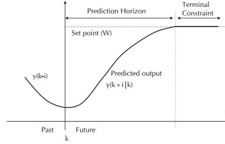
Fig. 1. CRHPC imposes an equality constraint.
