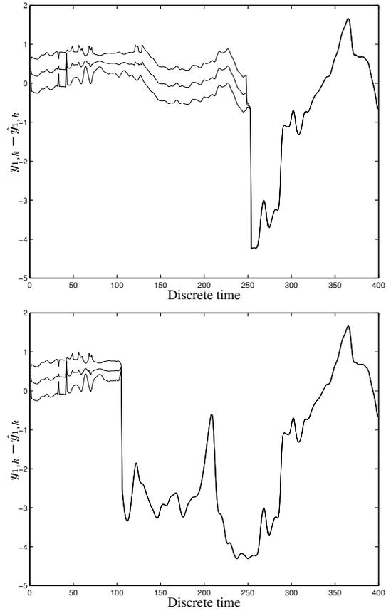
Fig. 1. A residual and its bounds for actuator faults: Case 1 (left), Case 2 (right).
