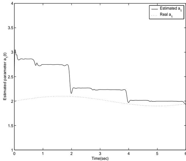
Fig. 4. Estimated time-varying parameter  $\hat{a}_1(t)$  (Solid-line:  $\hat{a}_1(t)$ ; Dashed line: real  $a_1(t)$ ).
