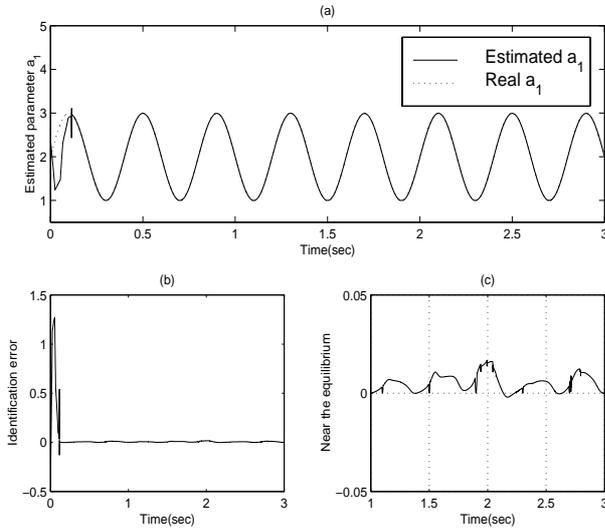
Fig. 1. Estimated *time-varying* parameter  $\hat{a}_1(t)$  and identification error: (a) Evolution of  $\hat{a}_1(t)$  (Solid-line:  $\hat{a}_1(t)$ ; Dashed line: real  $a_1(t)$ ); (b) Identification error of  $a_1(t)$ ; (c) Identification error near the equilibrium.
