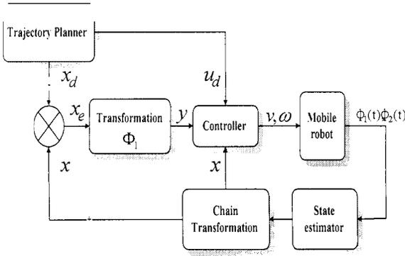
Fig 2 Block diagram of trajectory controller
