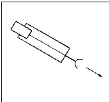
Fig. 2. Basic Braitenberg vehicle (one sensor, one motor)
