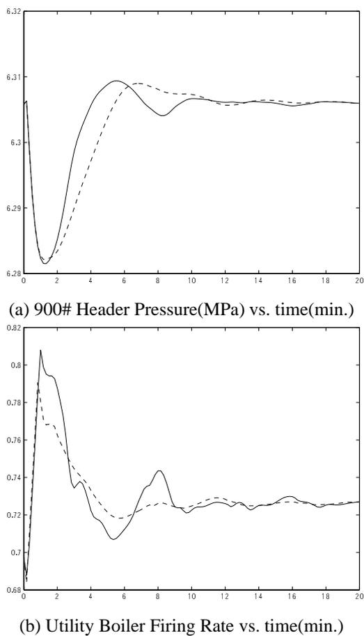
Fig. 4. Comparison of MPC and PID controllers for a 6.3kg/s steam demand change on the 900# header (solid: MPC; dashed: PID)
