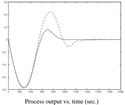
Fig. 3. MPC (solid) and PID (dash) control
