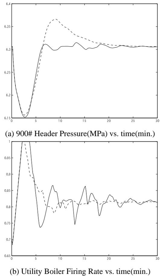
Fig. 5. Comparison of MPC and PID controllers for a 25.2kg/s steam demand change on the 900# header (solid: MPC; dashed: PID)
