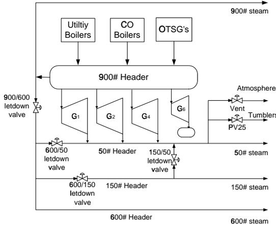
Fig. 1. A simple diagram of steam system in the Syncrude utility plant
