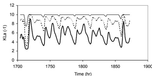
Fig. 5. (a) Control\_1; (b) Control\_3; (c) Control\_3 + equalisation tank. Variations of the oxygen transfer coefficient ( $K_La$ ) in the three aerated zones for  $J_{anox} = 6$ ,  $J_{aera} = 12$  with back-mixing: zone 1 (—), zone 2 (- - -) and zone 3 (—).
