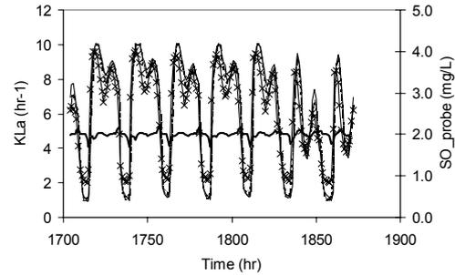
**Fig. 4. Variations of the oxygen transfer coefficient ( $K_L a$ ) in the third aerated zone for  $J_{anox} = 6, J_{aera} = 12$  without back-mixing (—), with back-mixing and  $\phi = 0$ , with back-mixing and  $\phi \neq 0$ . Comparison with  $K_L a$  of the original case ( $J_{anox} = 2, J_{aera} = 3$ ) (— $\times$ —) Dissolved oxygen at the probe level (—).**
