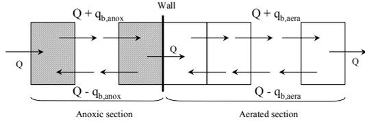
Fig. 2: Hydrodynamical model with a series of well-mixed tanks with back-mixing
