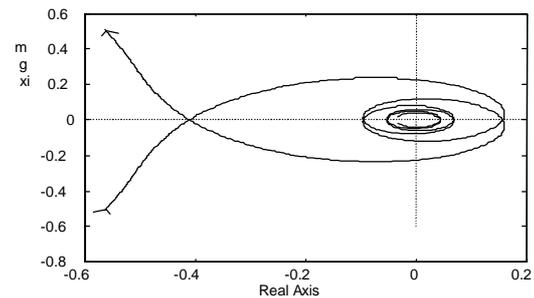
Fig. 6. Control response of the integrator with time delay (29) and the open loop Nyquist plot with the denominator approximation ( $m=0.3$ )
