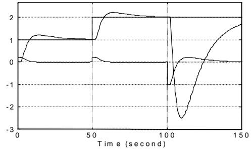
Fig. 5. Control response of the integrator with dead time (29) with neglecting of the dead-time ( $m=0.1$ )
