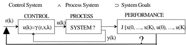
Fig. 6. A closed-loop system with system performance optimization rather than control performance optimization (Morel, 2001)
