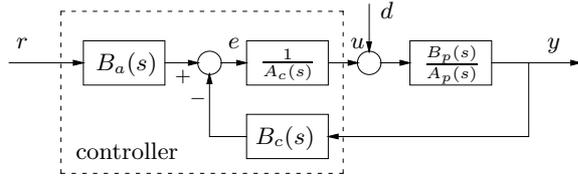
Fig. 1. Two-parameter configuration.
