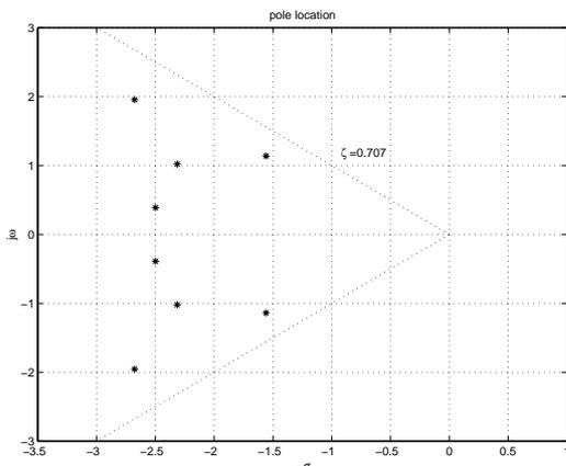
Fig. 5. Closed loop pole locations.
