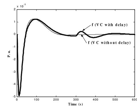
Fig. 6. Comparison of frequency control processes with different modes of VC.
