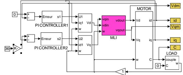
Fig. 3. Optimal torque control of a synchronous machine using a PWM technique
