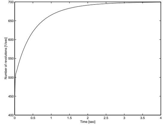
Fig. 4. Response of the number of revolutions of the closed-loop system (stable)
