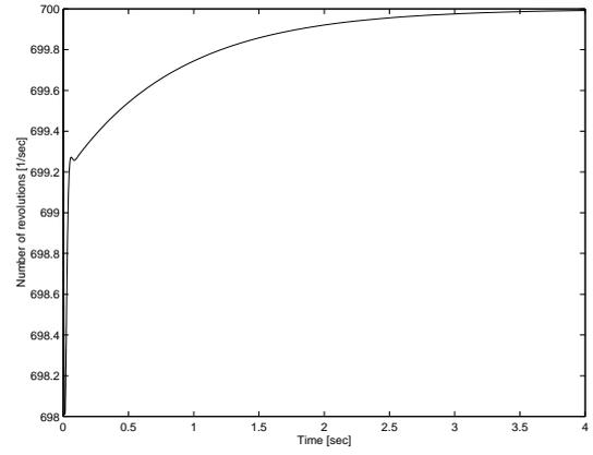
Fig. 5. Response of the number of revolutions of the closed-loop system (not sensitive)
