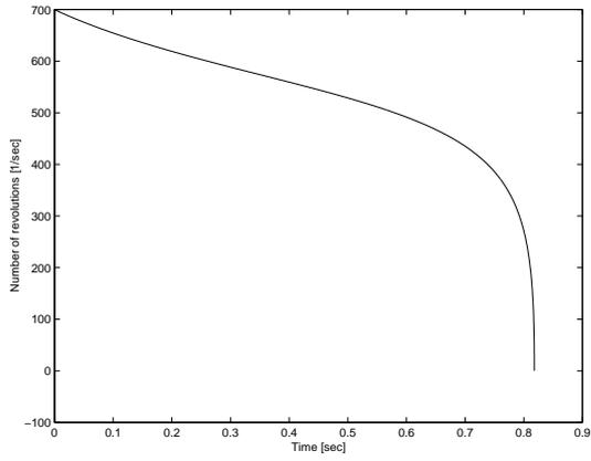
Fig. 3. Response of the number of revolutions of the open-loop system (sensitive)
