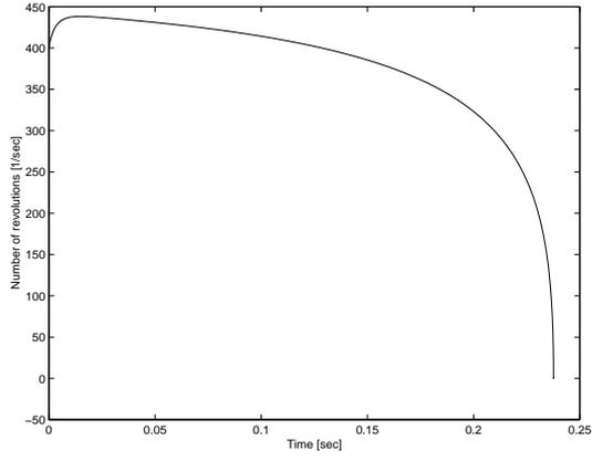
Fig. 2. Response of the number of revolutions of the open-loop system (unstable)
