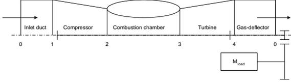
Fig. 1. The main parts of the gas turbine
