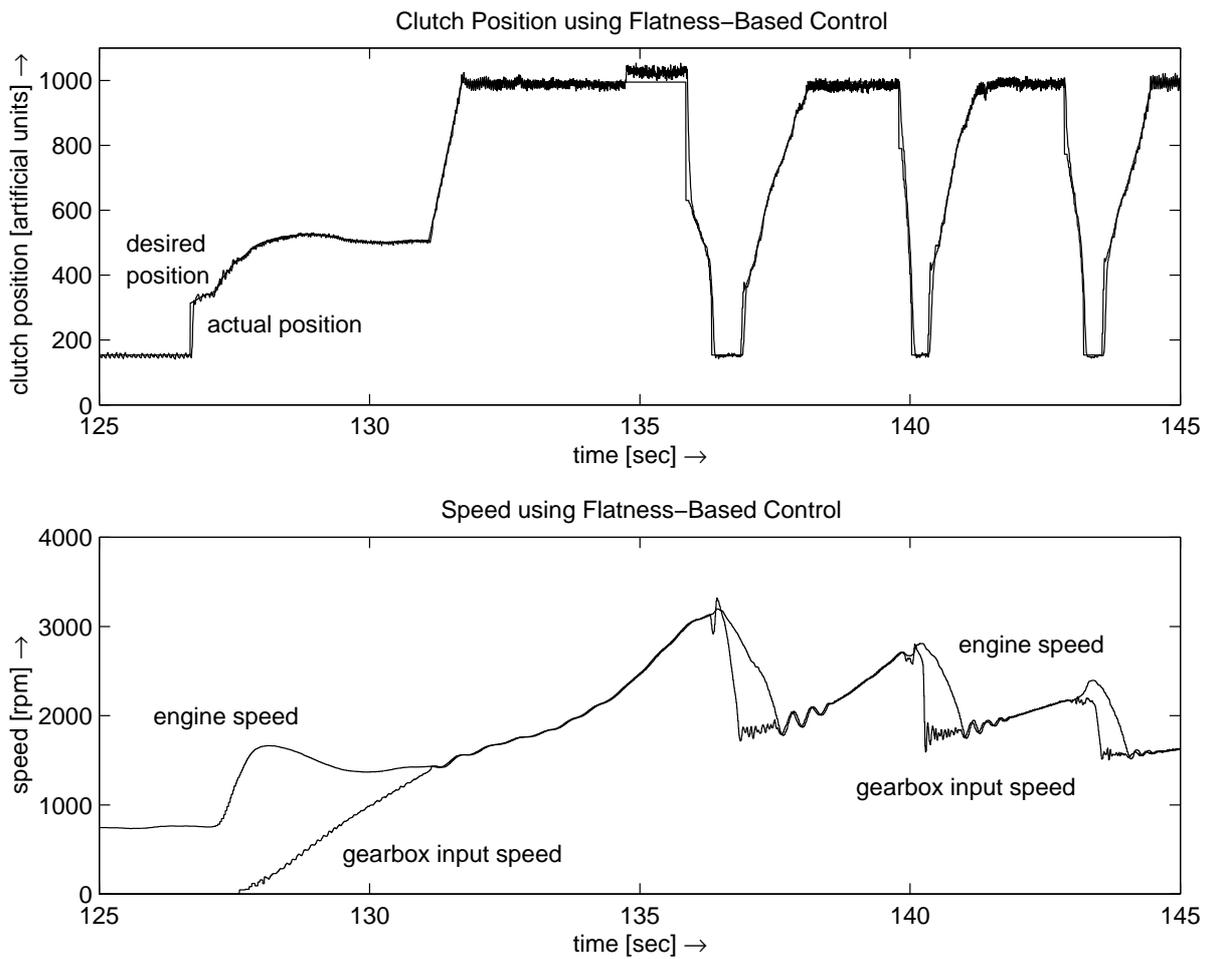
Fig. 5. Starting off and 1-2, 2-3, and 3-4 gear shifts using the flatness-based controller
