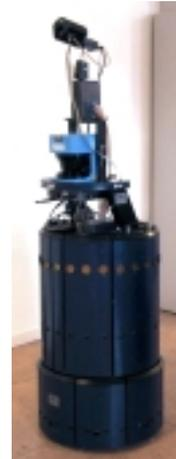
Fig. 6. B21 robot with a laser telemeter.
