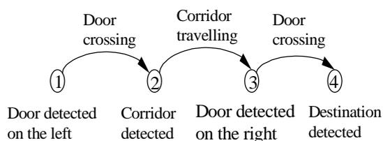
Fig. 2. Topological graph considered on the Navigation Chart.
