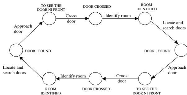
Fig. 3. Topological map for two adjacent nodes
