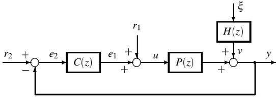
Fig. 1. Closed-loop system.
