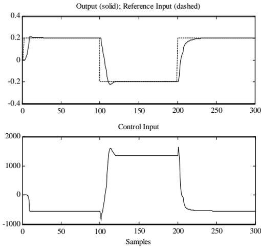
Figure 3: SDP-PIP-controlled closed loop responses.
