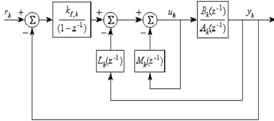
Figure 2: The Nonlinear SDP-PIP-controlled closed loop in feedback configuration.
