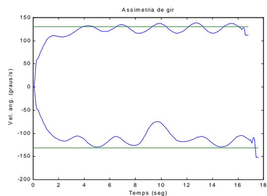
Fig. 4. Asymmetric dynamics between two wheels
