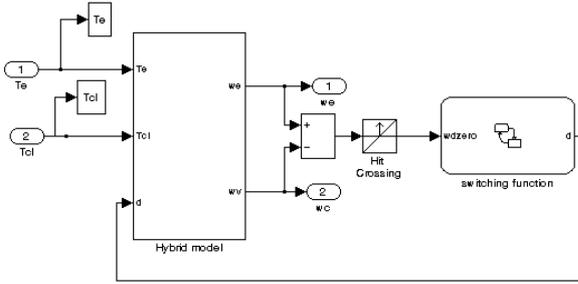
Fig. 2. Simulink scheme implementing the sixth order hybrid driveline model: the Stateflow "switching function" block discriminates between the slipping model and the engaged model.
