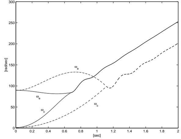
Fig. 3. Engine speed and clutch disk speed during the engagement; solid (dashed) lines correspond to the simulation under closed loop (open loop) control.
