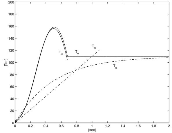
Fig. 4. Engine torque and clutch torque during the engagement; solid (dashed) lines correspond to the simulation under closed loop (open loop) control.
