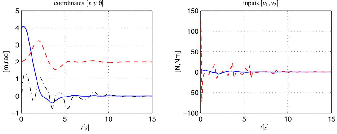
Fig. 2. V/STOL aircraft:  $x$  (solid),  $y$  (dashed),  $\theta$  (dash-dotted), inputs  $v_1$  (solid),  $v_2$  (dashed)
