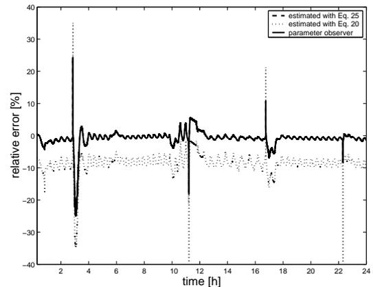
Fig. 7. Relative estimation-errors of the the mass flow observers
