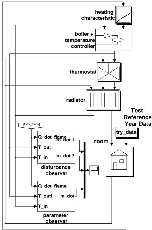
Fig. 5. Simulink model of the  $\dot{m}$ -observer
