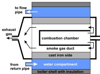
Fig. 2. Cross section of the boiler
