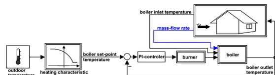
Fig. 1. Control of a central heating system
