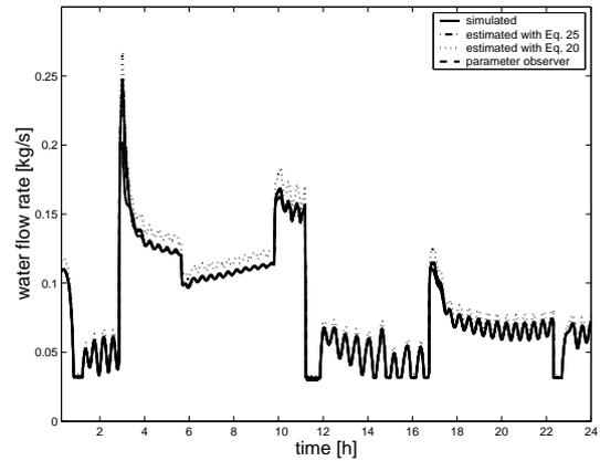
Fig. 6. Comparison of the results for the observer-based mass flow estimation-schemes
