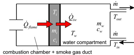
Fig. 3. Cross section of the simplified central heating furnace
