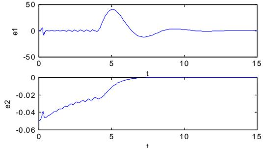
Fig2. errors of synchronization, the controller is taken on at  $t=4$ .  $e_1 = x_1 - \hat{x}_1, e_2 = x_5 - \hat{x}_5$
