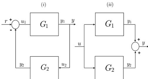
Fig. 1. (i) Feedback interconnection, (ii) Parallel interconnection.
