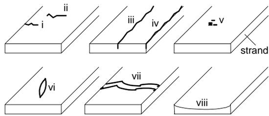
Fig. 2. Surface defects. i.) Transversal corner crack. ii.) Transversal center crack. iii.) Longitudinal center crack. iv.) Longitudinal off-corner crack. v.) Inclusions. vi.) Bleeder. vii.) Oscillation marks. viii.) Longitudinal depression.
