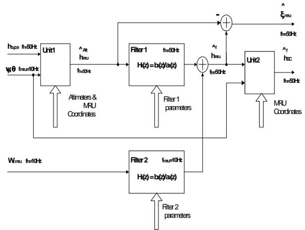
Fig.2. Algorithm structure for filtration of measurements of altimeters and vertical accelerometers.
