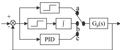
Fig.1 The structure of relay feedback based parameter identification method
