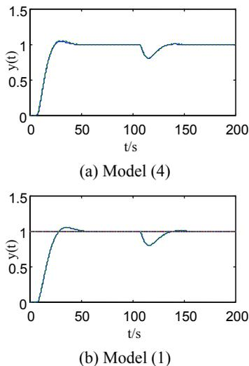
Fig.6 Response of the real process (solid line) and the low-order approximation model (dashed line) under the proposed PID/PI
