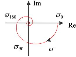
Fig.2 The Nyquist plot of the controlled object
