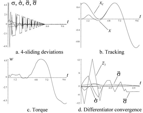
Fig. 4: 4-sliding control of the pendulum with an actuator
