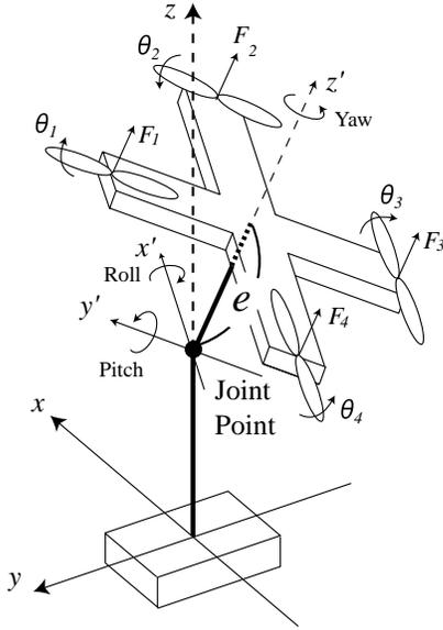
Fig. 2. Helicopter model fixed at a joint point.
