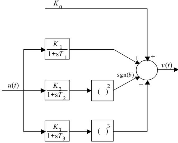
Fig. 1. Wiener model of first-order direction-dependent system
