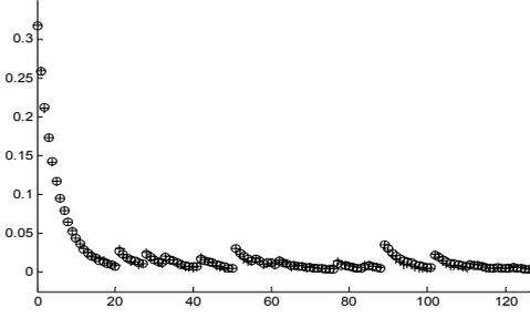
Fig. 2. Cross-correlation functions of first-order direction-dependent system (o) and Wiener model (+) with pseudo-random binary input
