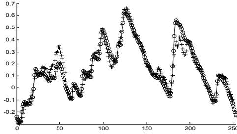
Fig. 6. Outputs of second-order direction-dependent system (equal gains) (o) and Wiener model (+) with inverse-repeat pseudo-random binary input
