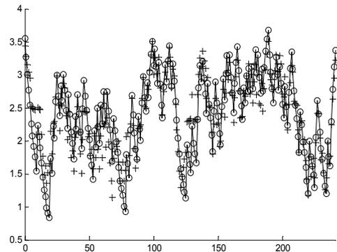
Fig. 5. Outputs of first-order direction-dependent system (o) and Wiener model (+) with inverse-repeat pseudo-random ternary input
