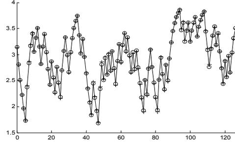
Fig. 3. Outputs of first-order direction-dependent system (o) and Wiener model (+) with pseudo-random binary input
