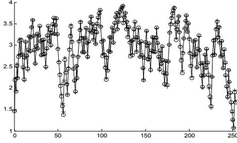
Fig. 4. Outputs of first-order direction-dependent system (o) and Wiener model (+) with inverse-repeat pseudo-random binary input
