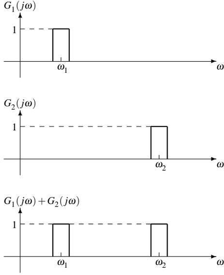
Fig. 5. The magnitude of  $G_1(j\omega)$  and  $G_2(j\omega)$ .
