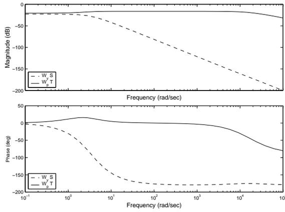
Fig. 6. The Bode plot of  $W_y S$  and  $W_p T$  with  $K = K_{GL_2}$ .
