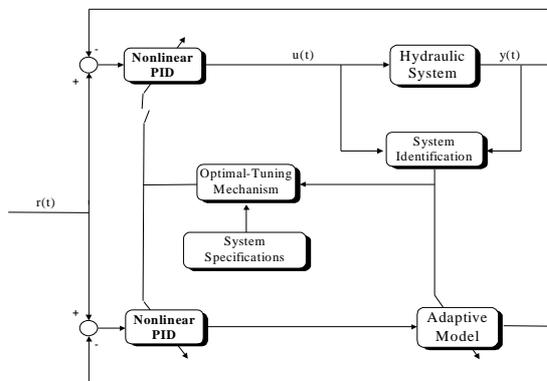
Figure 4 Optimal-tuning PID control scheme
