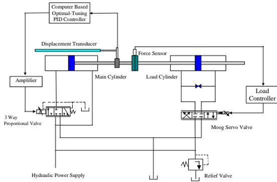
Figure 1 The hydraulic position control system
