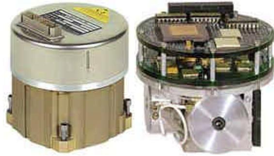
Fig. 2. The Litton LN-200 IMU.
