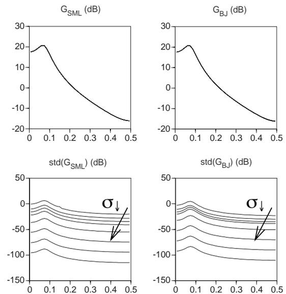
Fig. 4. Simulation results for a second order plant (eq.(20b): no model errors). Estimated plant and its sample standard deviation as a function of the normalised frequency for eight different values of the noise level:  $\sigma = 5, 2, 0.5, 0.1, 0.01, 0.001$  and  $0.0001$  (left: sample maximum likelihood, right: Box-Jenkins).
