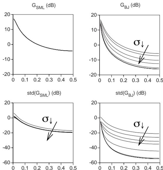
Fig. 3. Simulation results for a first order plant (eq. (20a): model errors). Estimated plant and its sample standard deviation as a function of the normalised frequency for eight different values of the noise level:  $\sigma = 5, 2, 0.5, 0.1, 0.01, 0.001$  and  $0.0001$  (left: sample maximum likelihood, right: Box-Jenkins).
