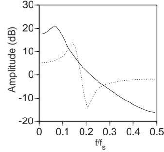
Fig. 2. True plant (solid line) and noise (dashed line) model.
