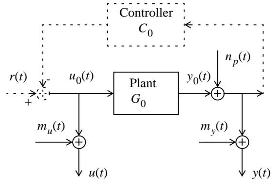
Fig. 1. Identification of a plant in open loop (solid line) or in closed loop (solid and dashed lines).  $r(t)$  is the reference signal;  $u_0(t)$ ,  $y_0(t)$  the input-output signals;  $m_u(t)$ ,  $m_y(t)$  the input-output measurement errors; and  $n_p(t)$  the process noise.
