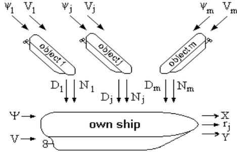
Fig. 7. Block diagram of a matrix model of game.
