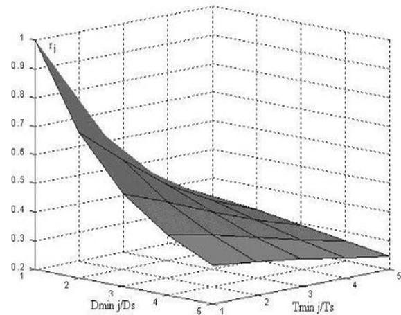
Fig. 8. The surface of the collision risk value  $r_j$  in dependence on relative values distance and time of  $j$ th object approach.
