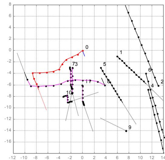
Fig. 6. The computer simulation of positional game trajectories in situation of passing 11 objects at the Kattegat Straits:  $D_s=1.5$  nm (nautical miles),  $t_k=6$  min,  $t_m=3$  min,  $r_j(t_k)=0$ ,  $d(t_k)=9.5$  nm.
