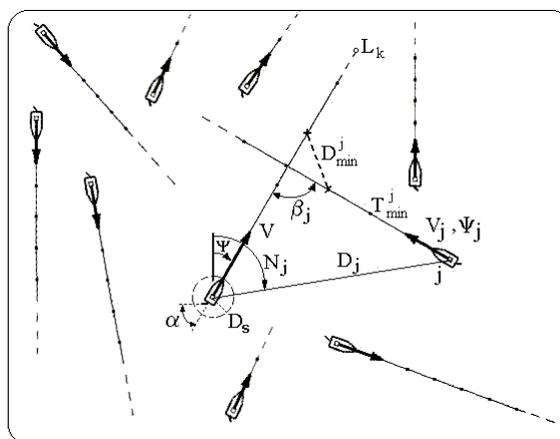
Fig.1. The process of the own ship passing  $j$  encountered objects.
