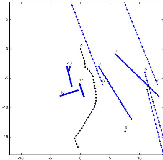
Fig. 9. The computer simulation of the own ship multi-step matrix game trajectory in situation of passing 11 objects at the Kattegat Straits for:  $D_s=1.5 \text{ nm}$ ,  $T_s=18 \text{ min}$ ,  $t_k=6 \text{ min}$ ,  $t_m=3 \text{ min}$ ,  $d(t_k)=6.31 \text{ nm}$ .
