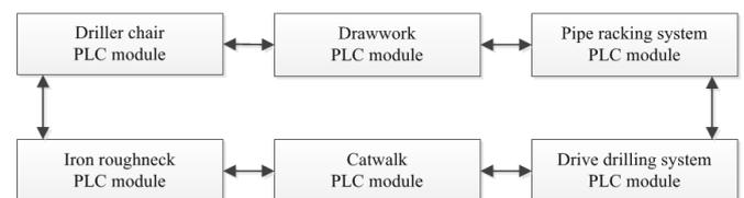
Fig. 4. PLC system network connection diagram.
