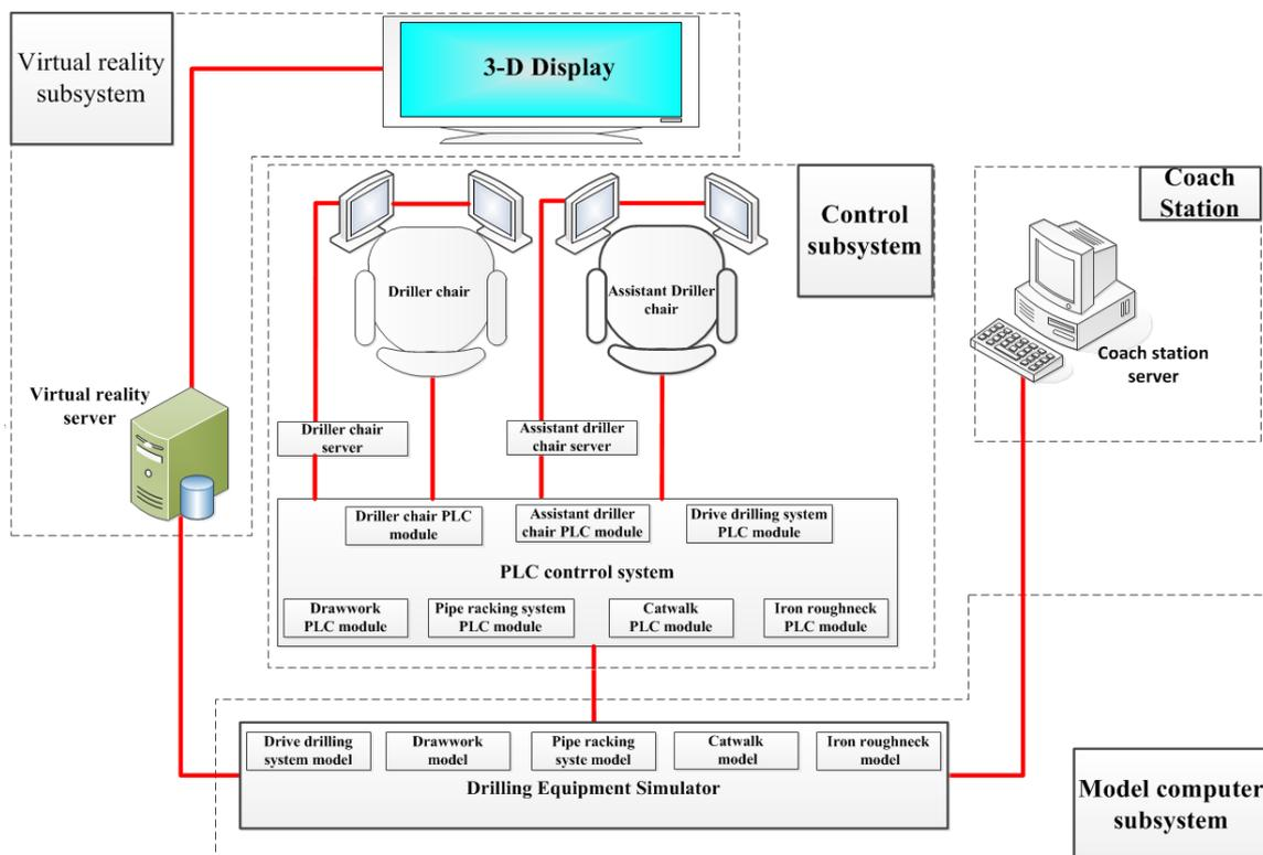
Fig. 2. Schematic diagram of simulation training system.
