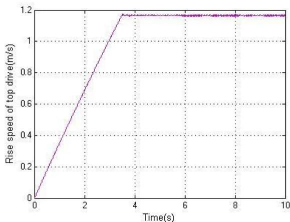
Fig.6. Rise speed curve of top drive under normal conditions
