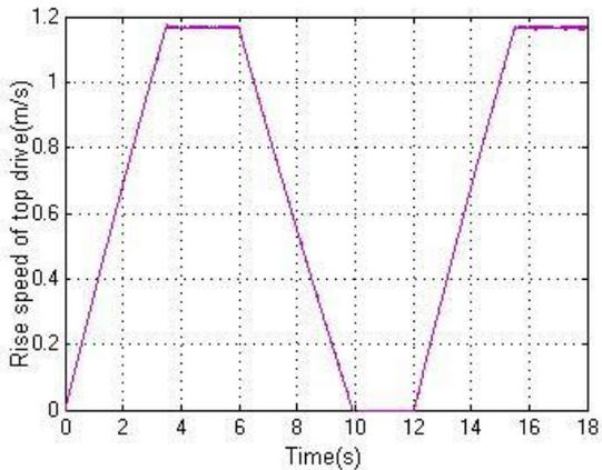
Fig. 8. Rise speed curve of top drive under fault conditions
