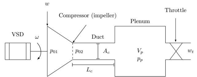
Fig. 2. The centrifugal compressor model.
