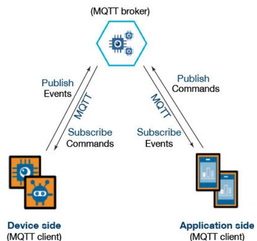
Fig. 1. MQTT Architecture
