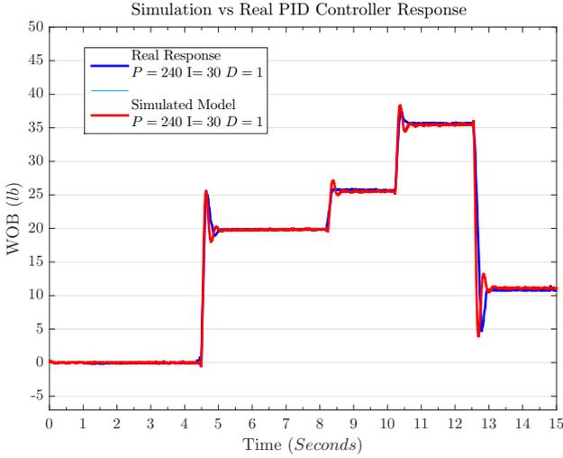
Fig. 5. Simulated vs actual response of the controller
