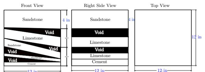
Fig. 2. Rock formations and structure used to validate performance, dips were introduced test the stability of the WOB controller
