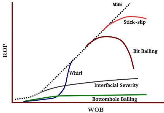
Fig. 3. Mechanical specific energy and its relationship to common drilling dysfunctions, adapted from Dupriest and Koederitz (2005)
