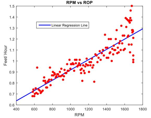
Fig. 6. Example of linear regression of the average rate of penetration as a function of revolutions per minute for a given homogeneous rock layer and constant drilling parameters
