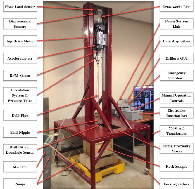
Fig. 1. Miniaturized drilling rig main components
