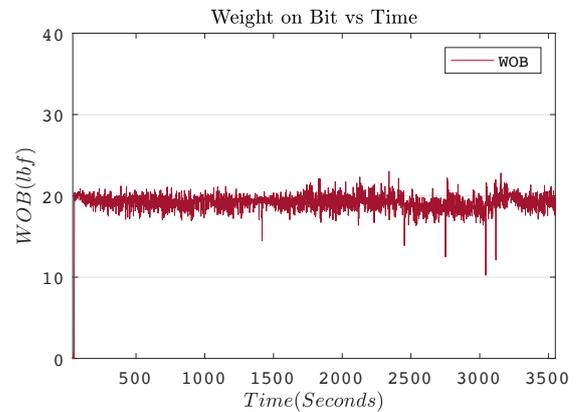
Fig. 7. PID controller performance while drilling
