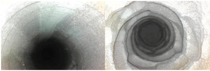
Fig. 8. Left: Dysfunction free borehole, Right: Severe borehole patterns caused by excessive bit whirl
