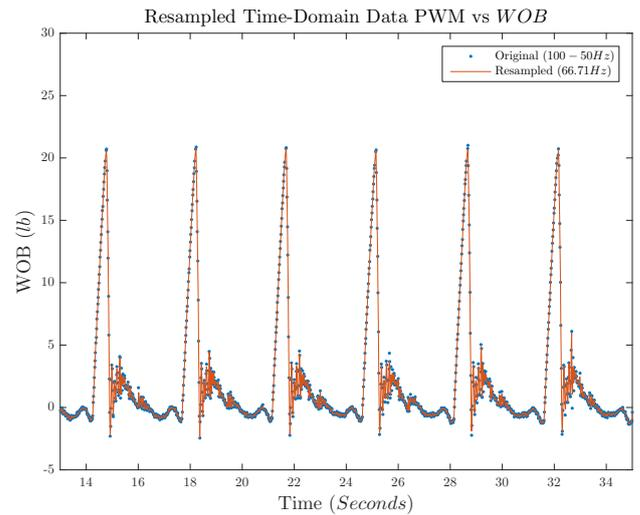
Fig. 4. Drawworks excitation response under steady state conditions.
