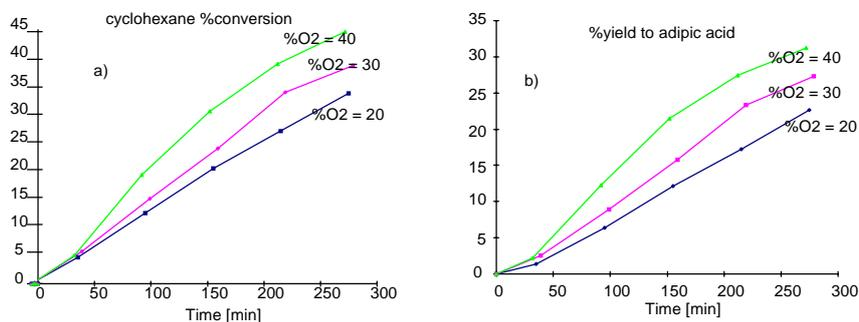
**Figure 3b.** Role of oxygen inlet mole fraction on: conversion of cyclohexane (left), yield to adipic acid (right). Time normalized setting is to zero at induction time.
