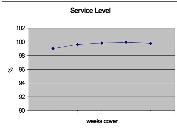
Figure 2. Variation of service level with finished goods safety stock for the collaborative case.
