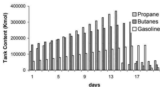
Figure 2. LPG tanks profiles in Natural Gas Plant II
