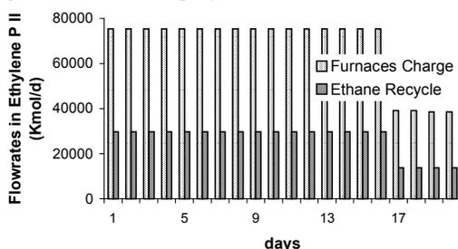
Figure 3. Ethane recycle and total furnaces charge profiles in Ethylene Plant II
