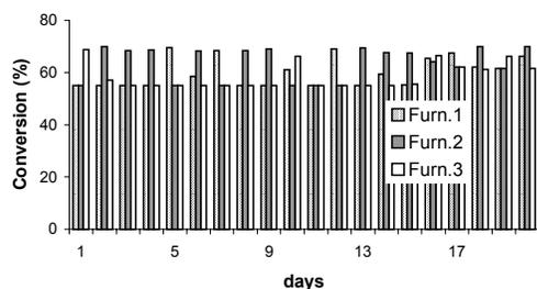
Figure 4. Conversion profiles in three furnaces from Ethylene Plant I
