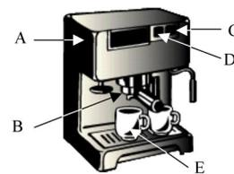
Figure 1. A typical espresso machine: (A) pressure vessel, (B) portafilter holding ground coffee, (C) on/off switch, with built in pressure indicator, (D) solenoid valve for espresso coffee, (E) cup holding espresso coffee.
