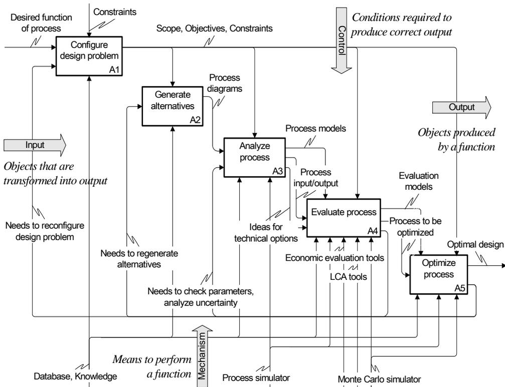
Figure 1. Overview of the whole process design activity: Design chemical process
