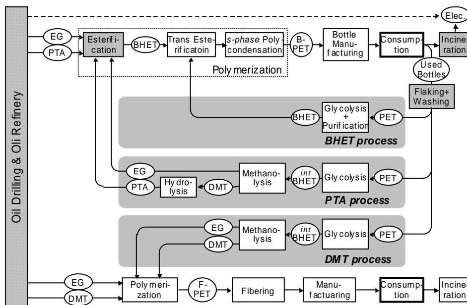
Figure 3. Life Cycle of PET products considering different chemical recycling processes. Int BHET represents intermediate state of BHET. Dark grey boxes indicate existing processes affected by the installation of process plants. Light grey boxes indicate chemical recycling processes.
